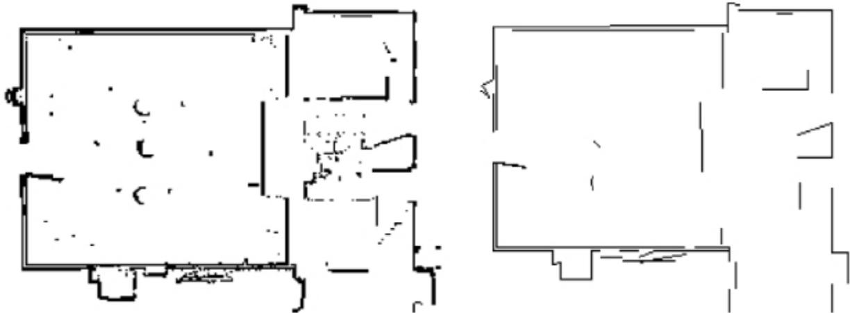
Figure 14: Maps consist of occupancy-grid points (left) and extracted lines (right).
